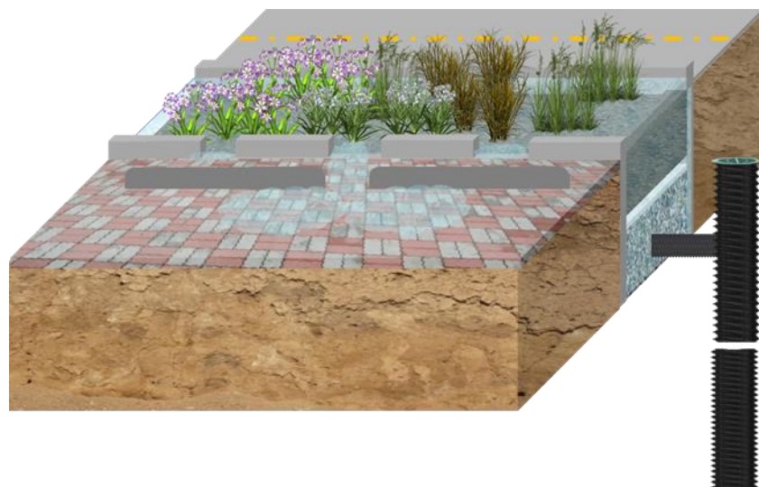
Stormwater Pretreatment Component—Curb Opening
