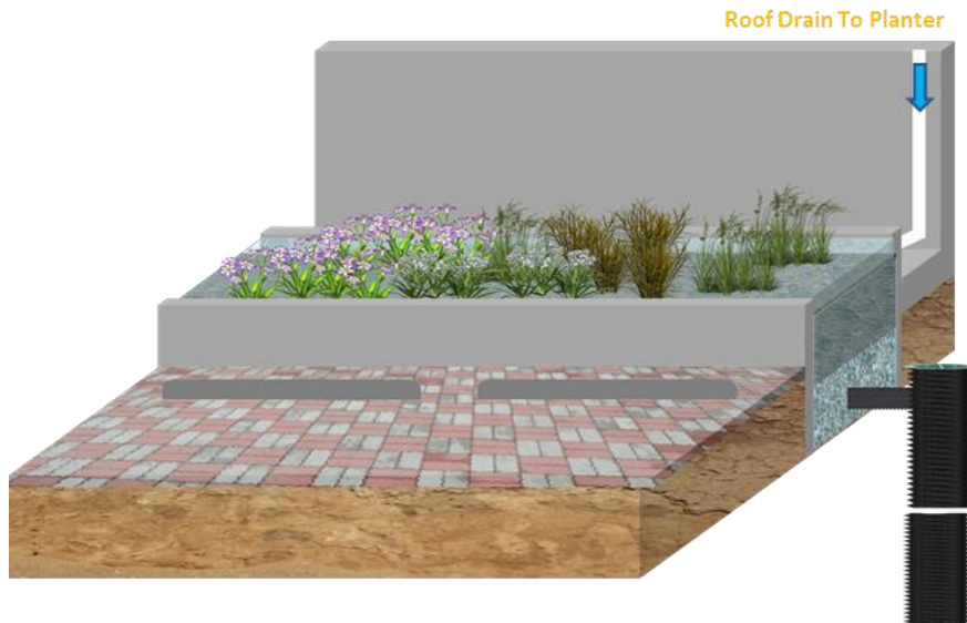
Stormwater Pretreatment Component—Roof Drain
